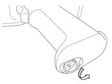
Figure 2-9-1 Installing /Replacing The Gun Grip Battery
