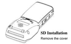
Figure 3-2 Installing SD Card
