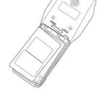
Figure 2-8-2 Installing /Replacing The Battery Pack
