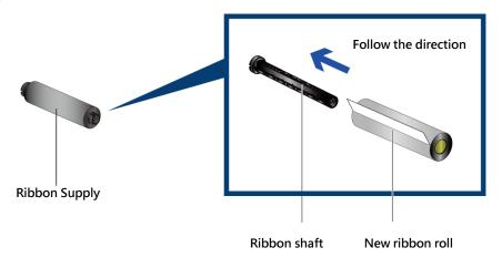
Install the empty ribbon core into ribbon shaft
