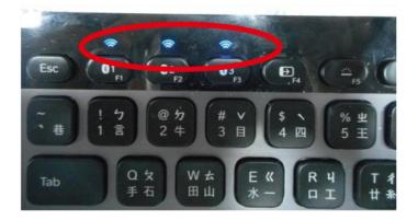
Step 3. The indicator will stop flashing if the Bluetooth keyboard connects to printer properly.
