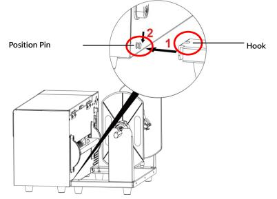
Step 2. Following the below arrow mark and direction to put the label roll into position.
