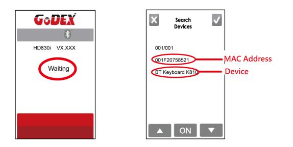
Step 7 . Press "ON" button on the LED panel to create a connection between the printer and the Bluetooth keyboard, and then the LCD panel will display " Please Enter PIN Code " .
