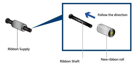
Install the empty ribbon core into ribbon shaft
