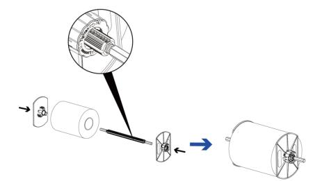
Step 3. Put the label roll into label roll stand.
