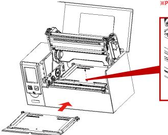
Press the print head hook on both sides to open the TPH
