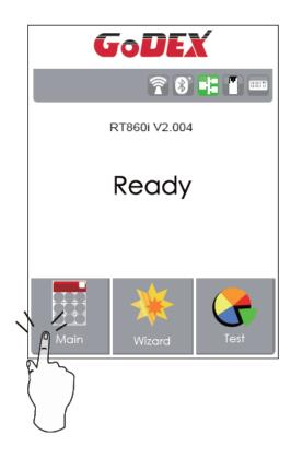
Tap the screen with your finger when you want to select on screen items such as settings icons. On the Ready Page, three function mode for setting. You can make various setting functions in FUNCTIONAL MODE.
