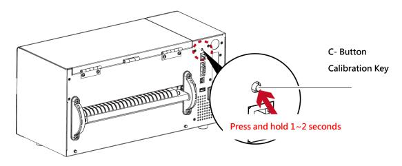
Press and hold the <sup>r</sup>C-Button <sub>J</sub> around 2 seconds, the printer will run the media calibration
