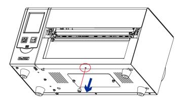
Step 1. Disassemble the bottom case screws (Marked in Red circle)
