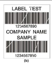
2. To keep track of the change in print quality, you should adjust the screws by half a turn at a time. Print a test page. If there is no improvement in the print result, turn the screw by another half turn. Do not turn the adjustment screw more than two full turns.
