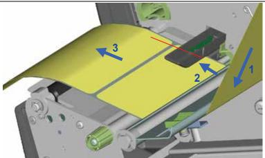
The labels pass between the wall of the printer housing and the adjustable paper guide.
