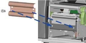
4. Installation of the rewinder guide is now complete.
