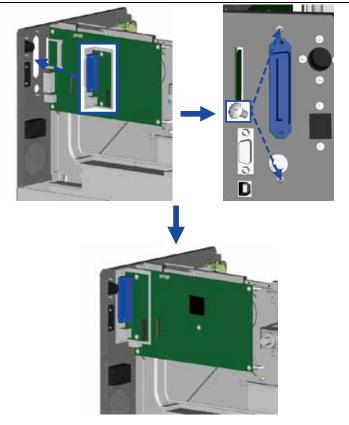
Connect the 30-pin connection cable to the motherboard.
