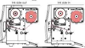
5. Pass the ribbon under the print head and back up on the other side. Attach it to the empty ribbon core.
