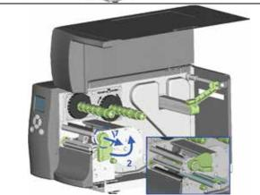
When using a variety of label stock and ribbons, the ink may not be evenly distributed. If there is no printed image on one side of the paper, or the ribbon wrinkles, the print head pressure must be readjusted using the TPH spring boxes.
