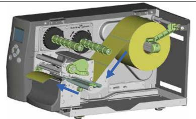
8. Pass the label stock through the sensor and up to the tear-off plate.
