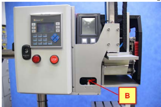
Picture 3: Valve to set the airflow through the label blow-on nozzles
