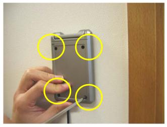
5. Once the wall mounting step is finished, place the PVC sticker on to the front casing to cover the screw holes.
