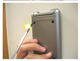
4. Tighten each screw to fix the ACR120 reader on the wall.
