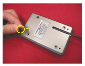
3. Drive in the screws into the specified holes for wall mounting.
