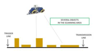
2D PackTrack is Matrix software algorithms that solve sorting applications over conveyors where carton, parcels, or packages are close to one another, i.e the gap between cartons is small and the code position is random throughout the scanning area.
