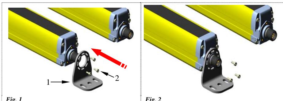
Orient the bracket according to the desired rotation angle, ensuring that the slots correspond to metal inserts on the cap. Use an allen key to tightly fix the screws (2).
