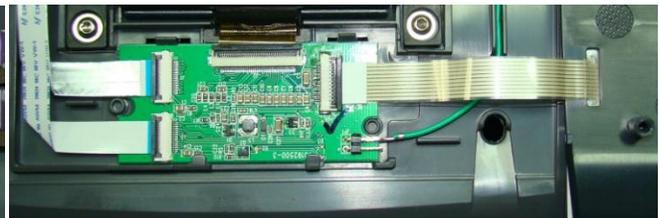
Flex used on LCD printers
