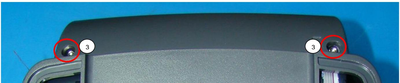
Installation is reverse order of removal. Ensure all cables and wires are routed correctly, and none of them are pinched or stressed by the lower frame cover. Torque the fasteners to 3.4 +/- 0.4 in-lb or 4.0 +/- 0.5 kgf.cm Use the final test procedure noted in the OTPPCX3-000 PC23 AND PC43 PRINTERS FINAL TEST.
