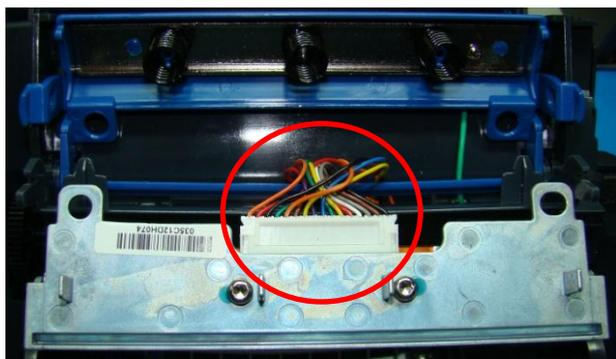
Installation is reverse order of removal. When re-installing the Printhead assembly in the Printhead tray ensure both sides of the assembly have been fully inserted in the tray, and the back part of the assembly is lined up with the two alignment pins. Refer to the picture in step 3 for an example of proper part alignment. Install blank receipt or label stock and print quality labels as detailed in the PC23 and PC43 Desktop Printer User Manual.
