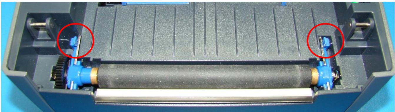
Installation is reverse order of removal. When re-installing the platen roller assembly ensure the drive gear is fully seated, and the blue latches are locked in the down position.
