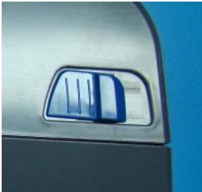
2. Gently push outward on the two blue latches and pull them towards the front side of the printer. Remove the platen roller assembly.
