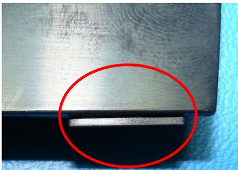
Tab found on the printers with the USB port on the front.
