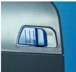
2. Remove the two blue buttons from the top cover frame. Gently press down on the buttons tab on the inside of the top cover to remove them.
