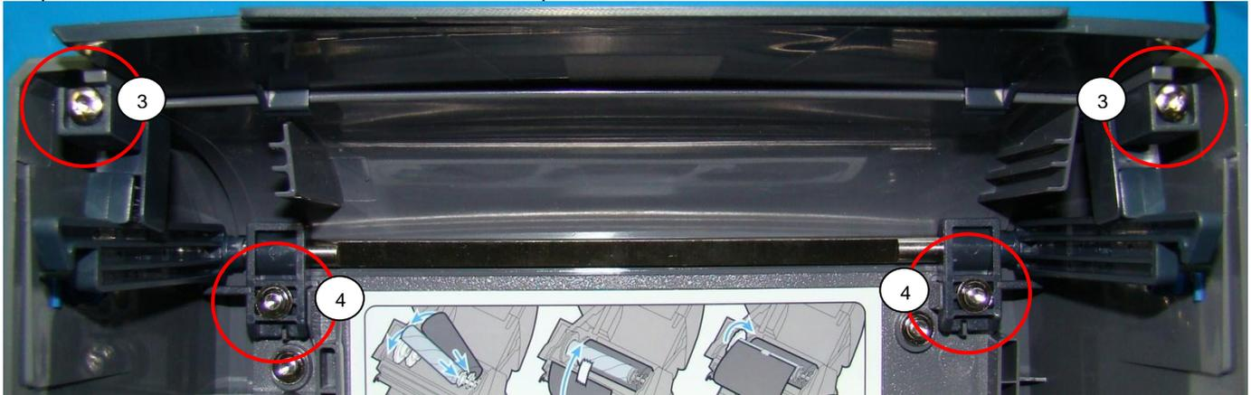
Installation is reverse order of removal. During installation of the latches ensure the spring is fully captured and engaged over the pin on the latch arms. Refer to the below picture for proper spring position. Torque the fasteners to 3.9 +/- 0.4 in-lb or 4.5 +/- 0.5 kgf.cm.
