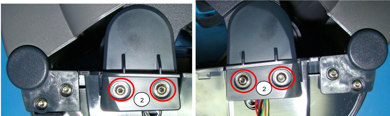
Installation is reverse order of removal. Torque the fasteners to 3.9 +/- 0.4 in-lb or 4.5 +/- 0.5 kgf.cm Use the final test procedure noted in the OTPPCX3-000 PC23 AND PC43 PRINTERS FINAL TEST.
