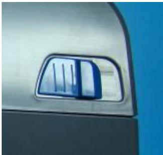
2. Gently push outward on the two blue latches located in the TTR assembly on both sides of the Printhead assembly. The Printhead tray will drop down.
