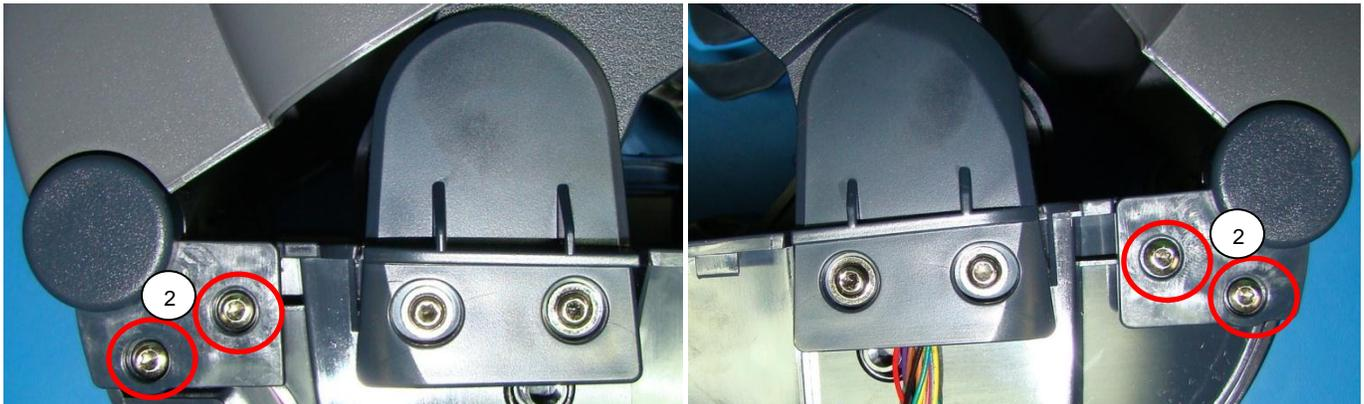
Installation is reverse order of removal. Ensure all wires and cables are routed as pictured below. Torque the fasteners to 3.9 +/- 0.4 in-lb or 4.5 +/- 0.5 kgf.cm Use the final test procedure noted in the OTPPCX3-000 PC23 AND PC43 PRINTERS FINAL TEST.
