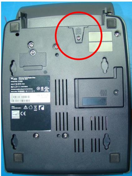
Installation is reverse order of removal. Torque the fastener to 1.3 +/- 0.4 in-lb or 1.5 +/- 0.5 kgf.cm Use the Ethernet test procedure noted in the OTPPCX3-000 PC23 AND PC43 PRINTERS FINAL TEST.
