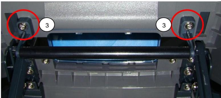
Installation is reverse order of removal. The brackets are keyed to tabs in the top frame. Torque the fasteners to 3.9 +/- 0.4 in-lb or 4.5 +/- 0.5 kgf.cm.
