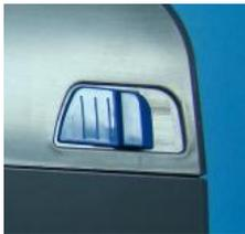
2. Gently pull up on the front cover to remove it from the printer's lower housing.
