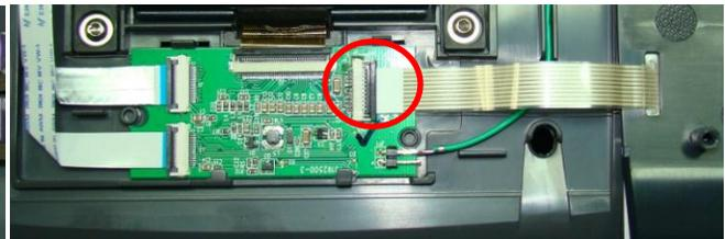
Control panel flex used on LCD printers
