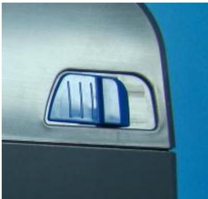
2. Gently push down on the media window's release tabs, and then push the window out towards the backside of the printer.
