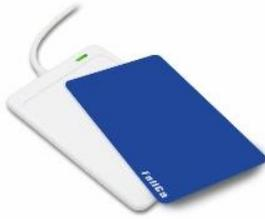
It is a PC-linked Contactless Smart Card Reader/Writer developed on the 13.56MHz Contactless Technology. It is the world's first CCID Compliant Contactless Card Reader/Writer that follows both ISO14443 and ISO18092. This device is designed to support not only MiFara and ISO14443 Type A and B Cards but also FeliCa and NFC tags.
