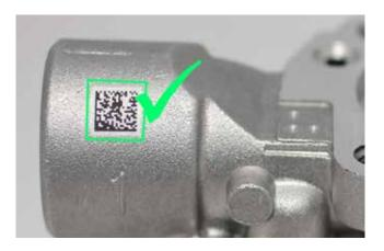
LIGHTER Suite combines into an unified GUI (Graphical User Interface) a powerful vectorial graphical editor, an advanced laser controller and the innovative MARVIS™ (MArk Read Verify Integrated Solution) feature to seamless interact with AutoID code reader for in-line validation of marked traceability codes. MARVIS™ connects any Datalogic MATRIX
