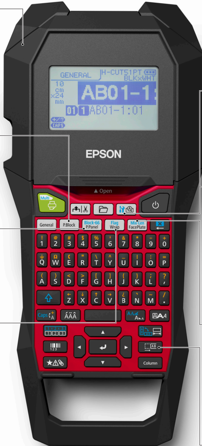
Flag & Wrap Creates cable flags and self-laminating overwraps for easy identification of labels.
