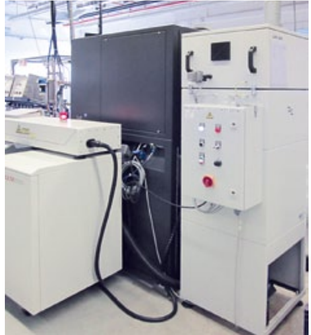
Laser welding system with integrated extraction and filtration system
