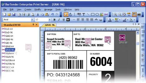
Simply drag desired RFID objects to anywhere on the label. (Since RFID objects never print, they display next to the label.)
