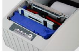
Dentiform belt driving mode print head
