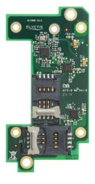
As an option, a secondary board offers an extension of two additional SAM slots.
