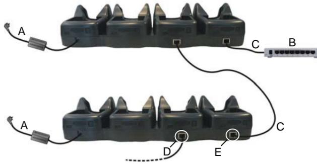
Figure 7 - Daisy chaining Ethernet Connection
