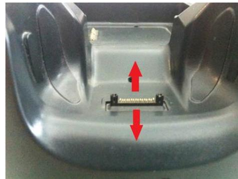
4. Use a dry cloth to remove any dirt near the contacts area and to clean the plastic parts. If the plastic parts of the equipment are very dirty, slightly dampen the cloth with only water.
