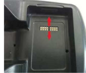
4. Use a dry cloth to remove any dirt near the contacts area and to clean the plastic parts. If the plastic parts of the equipment are very dirty, slightly dampen the cloth with only water.
