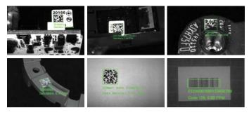
1DMax with Hotbars technology deliver high-speed reading of damaged or poorly printed 1-D barcodes as small as 0.8 pixels per module (ppm).
